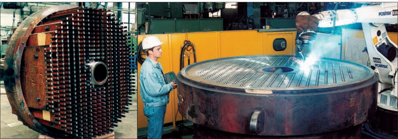
Automatic welding of stiffener fingers to tubesheet with robot
