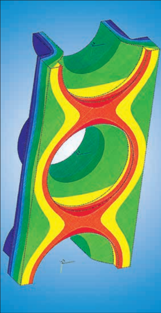
Fig. 26: Temperature distribution of tube inlet section by finite element analysis
