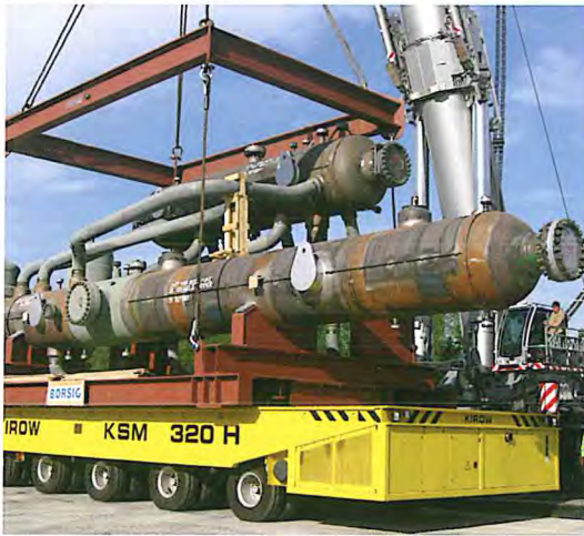
A waste heat recovery system being shipped.
