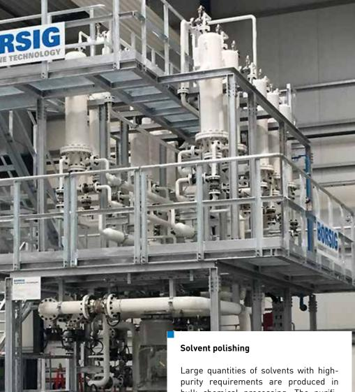
purity requirements are produced in bulk chemical processing. The purification of solvents from small amounts of substances with a higher molecular weight by rectification is an energyintensive and therefore sometimes uneconomical process.
