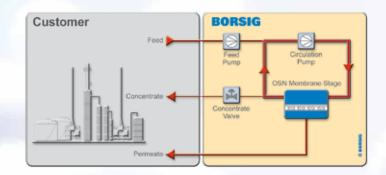
OSN Units are operated in cross-flow mode either batch-wise or continuously according to the application.
