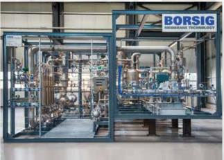
the nitrogen before it is fed back to the suction side of the vent recovery compressor.
