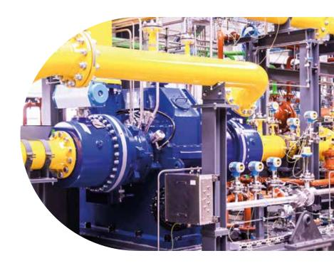
With more than 60 years of expertise in turbo compressor construction, BORSIG ZM Compression GmbH offers integrally geared centrifugal compressors according to customer specifications as turnkey solutions with all necessary system components.
