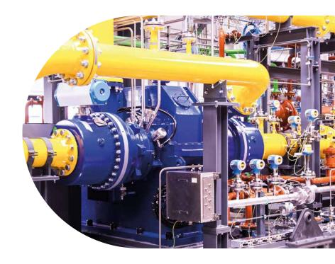
With more than 60 years of expertise in turbo compressor construction, BORSIG ZM Compression GmbH offers integrally geared centrifugal compressors according to customer specifications as turnkey solutions with all necessary system components.
