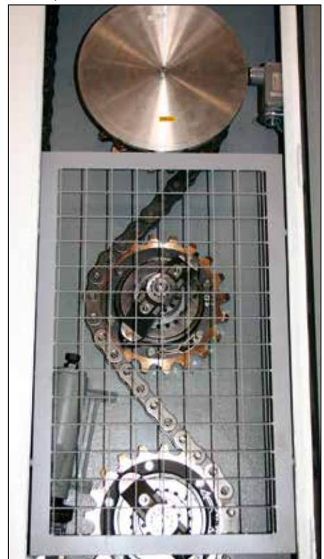
Touch protection, rotation sensor
