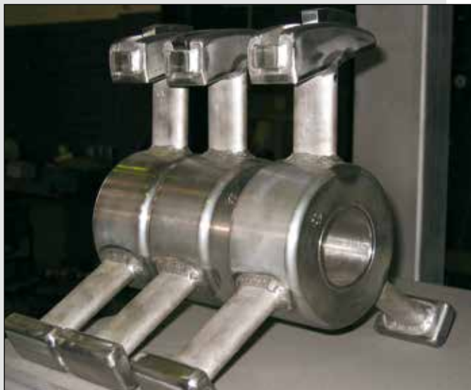
Spider supports for acetylacetat service
