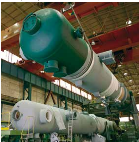
BORSIG process gas waste heat boiler
