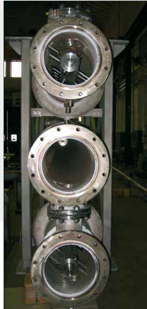
Installed scraper shaft
