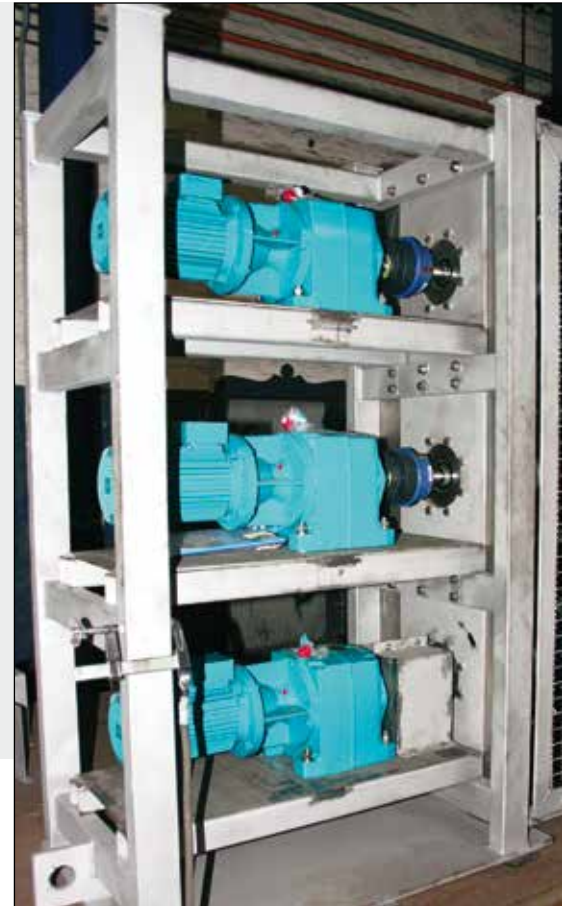
Gear motors for drive system
