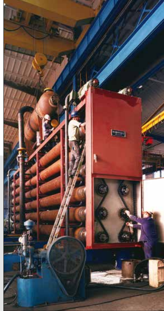
BORSIG scraped surface exchanger in the workshop
