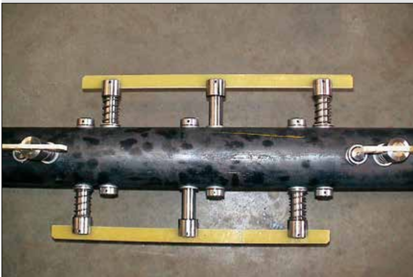
Replacement scraper shaft for paraxylene service
