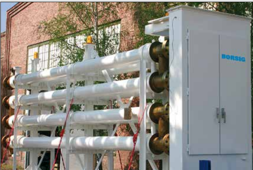
Scraped surface exchanger for fatty acid service
