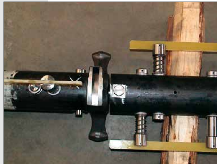
Assembled scraper shaft with spider support
