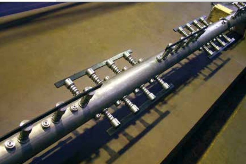
Assembled scraper shaft for acetylacetat service
