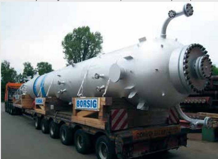
BORSIG synthesis gas cooler downstream of partial oxidation ready for dispatch
