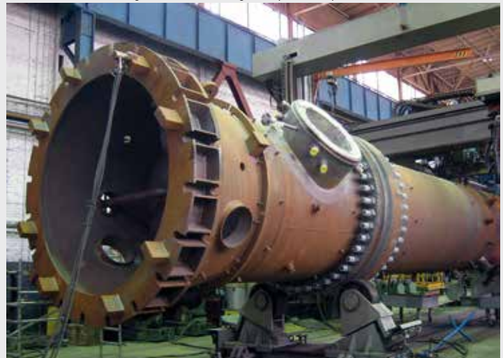
Robot flame-cutting of vessels and large components up to 4,000 mm diameter
