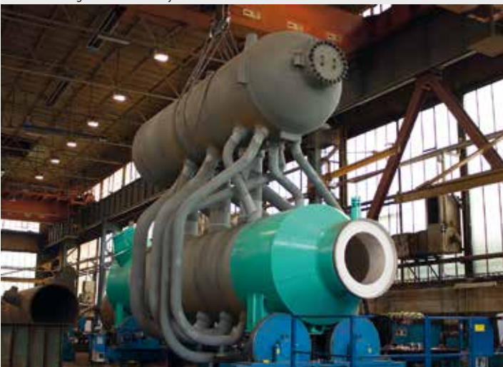
Process gas waste heat system
