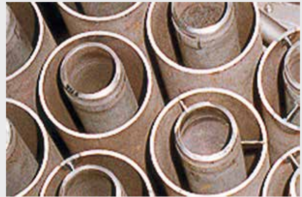
Assembly of connecting pipes and double tubes
