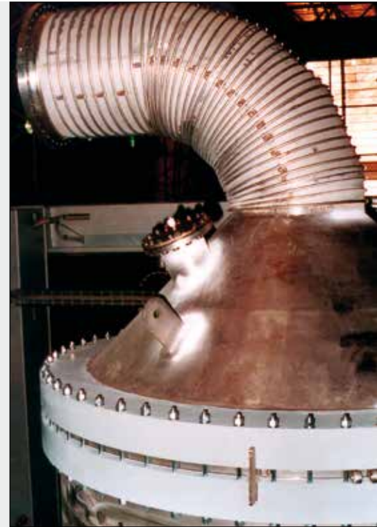
Upper head for waste heat boiler for formaldehyde plants
