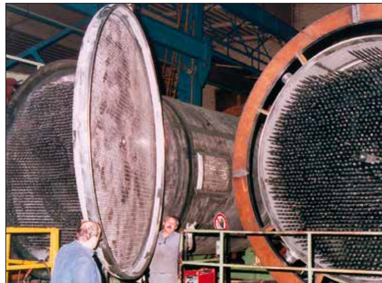
Installation of lower tubesheet for a fire-tube boiler
