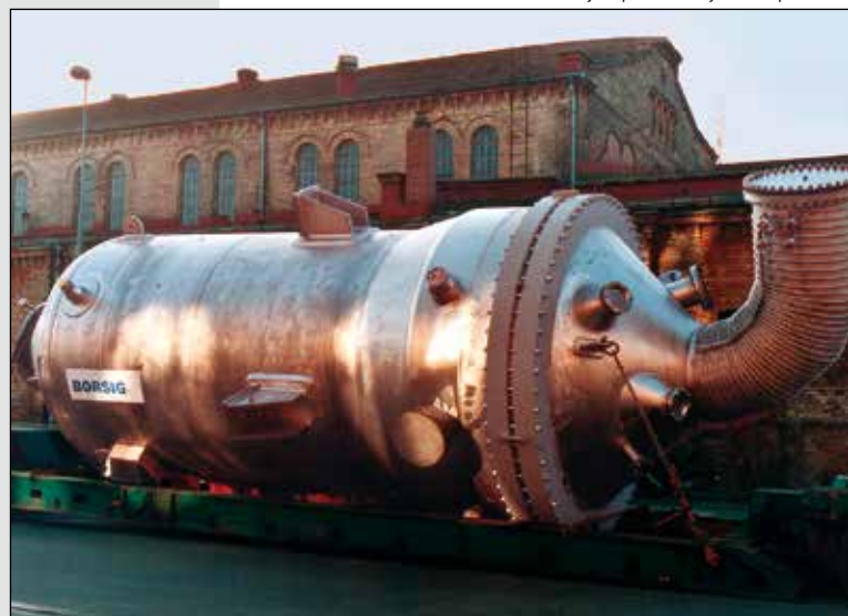
Waste heat boiler for a formaldehyde plant ready for shipment
