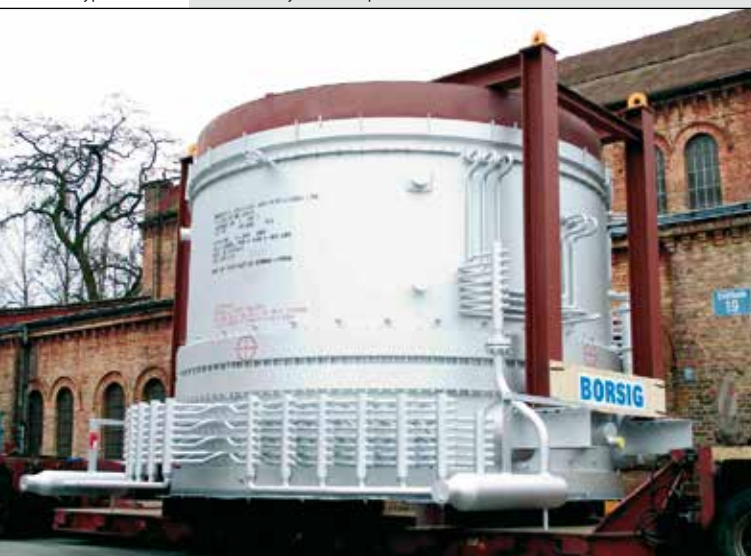
LaMont type waste heat boiler ready for transport
