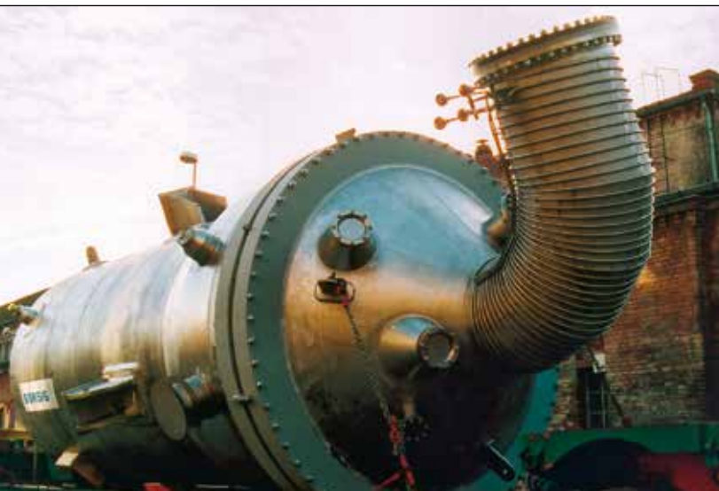
Reactor/waste heat boiler for formaldehyde production
