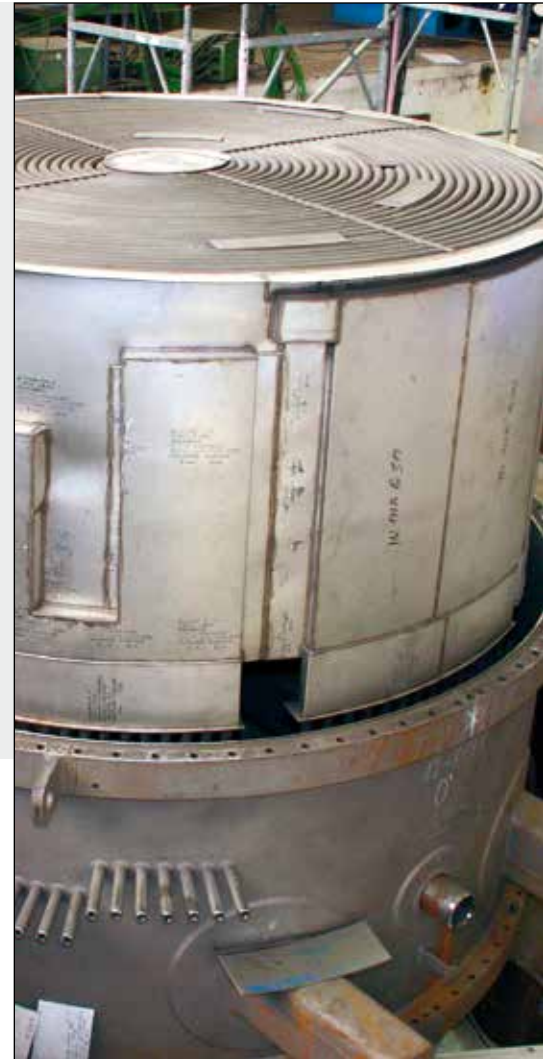
Completed metal shroud and tube bundle
