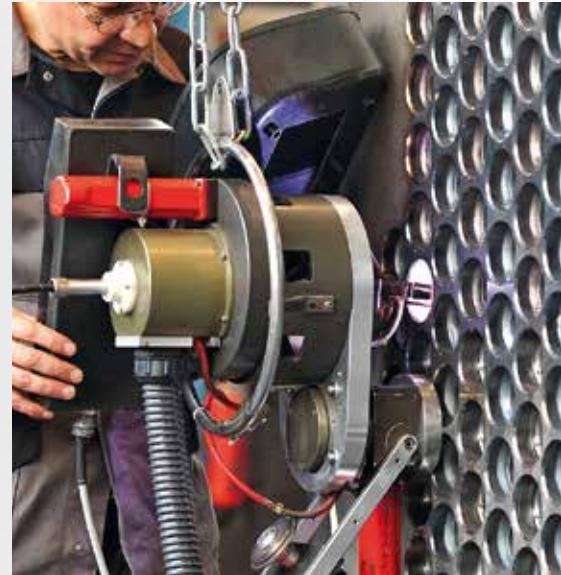
Automatic full penetration tube to tubesheet welding
