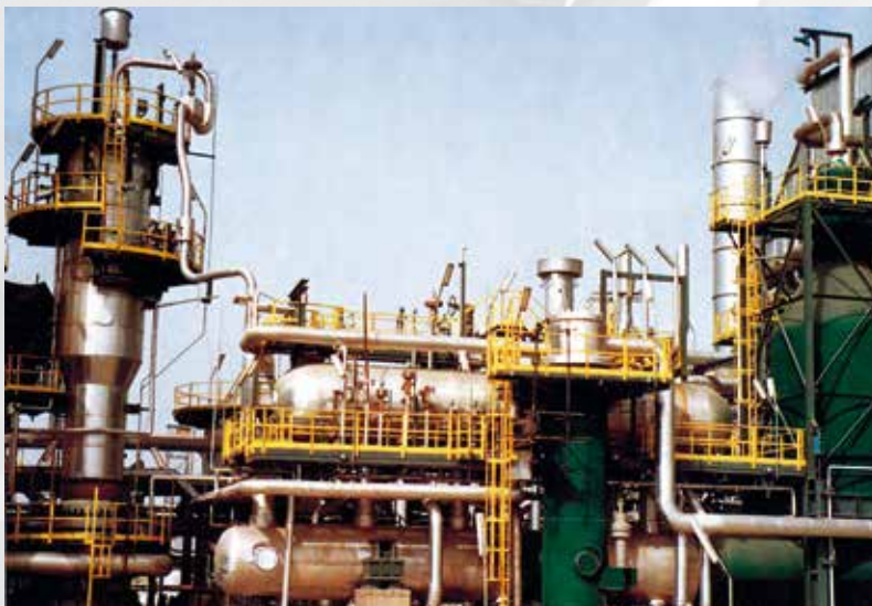
Ammonia plant with synloop WHB, reformed gas WHB, steam superheater and steam drum
