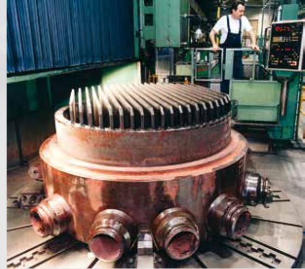
Machining of stiffened tubesheet system
