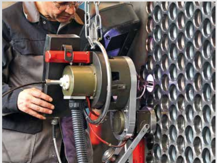
Automatic full penetration tube to tubesheet welding
