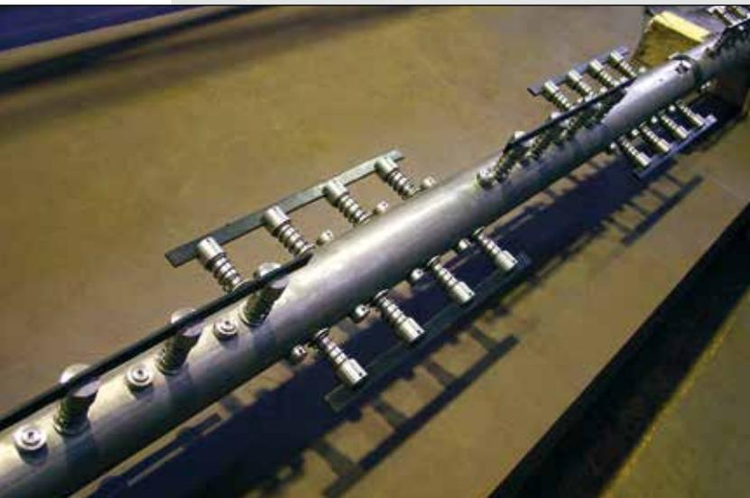
Assembled scraper shaft with spider support
