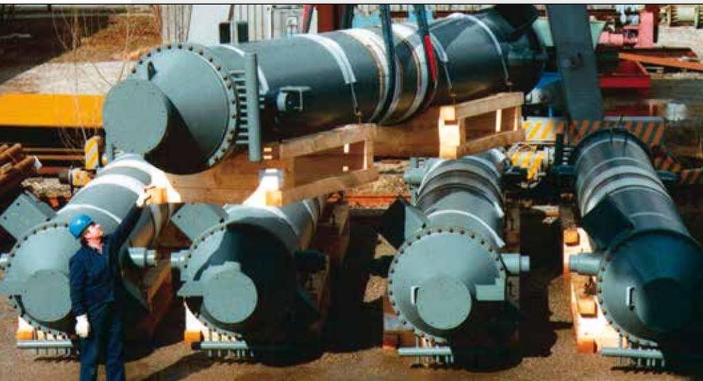
BORSIG linear quencher (BLQ) for ethylene cracking furnaces
