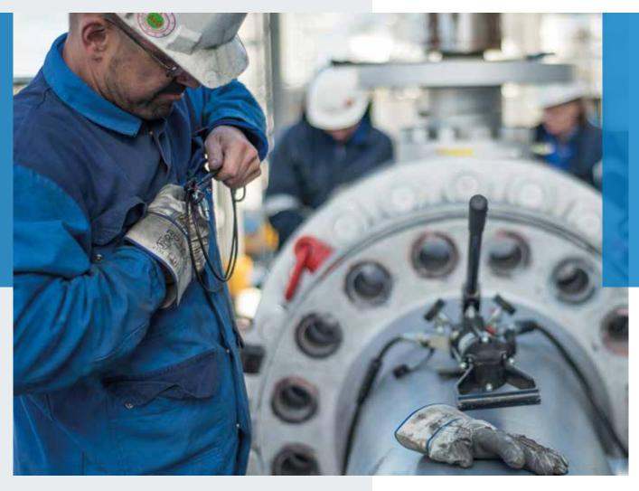
Valves severely damaged by corrosion are refurbished by cladding and hardfacing sealing surfaces including respective PWHT measures in such a way that they are equivalent to new fittings.
