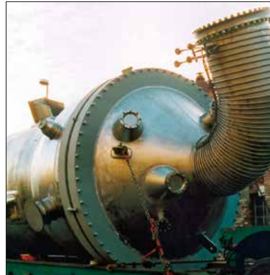
Transport of a waste heat boiler for a formaldehyde plant
