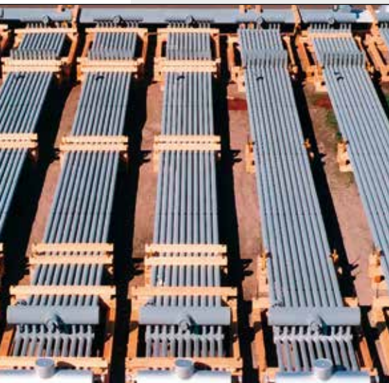
BORSIG linear quencher (BLW) for ethylene cracking
