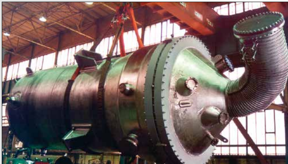
Waste heat boiler for formaldehyde ready for shipment
