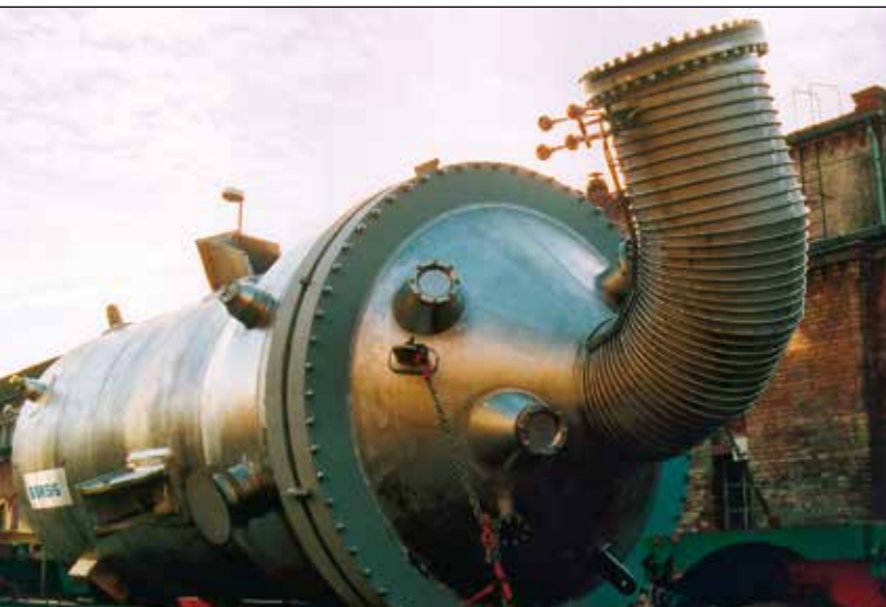
Reactor/waste heat boiler for formaldehyde production
